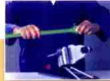
Step 4 : Remove the pipe and fitting from the dies and immediately push the pipe into the socket and allow it to cool.
